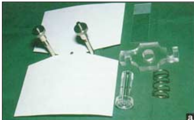
Figures 5a and 5b Sayk sedimentation chamber (modified by Kölmel). Filter paper is put onto an object slide lying on a floor plate. In the middle of the paper there is a hole 5–12 mm in diameter. A hollow cylinder with exactly the same inner diameter as the hole is placed on top. A spring and plate exert downward
