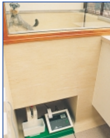
Figure 2 The WCPN canine urine pH monitoring system.
